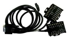
**DB26** can provide stable 12V/2A , 5V/1 and GND connection for external devices and it includes 2 boxes. I/O alarm box is a device designed for Mobile Digital Video Recorder (ViPRO MVR series), providing the I/O interface of alarm input, alarm output and speed, to realize the functions of alarm test and alarm linkage, etc. RS232/485 wiring box integrates the interface of RS-232, RS-485 and so on, to realize the serial communication between the external device and Mobile DVR.
